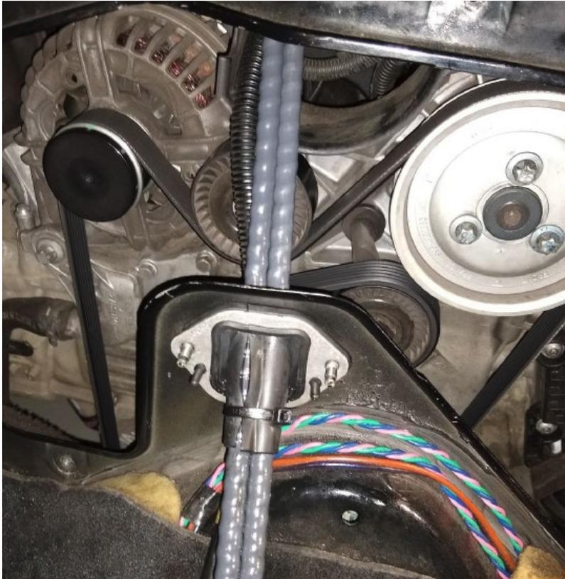
**#11. Connect the cables to the transmission brackets and tighten the nuts. I always apply some grease to the threads. Do not connect the rod ends just yet.**
