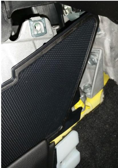
**The right panel will have the 12v power source. You can leave it connected and just lay it to the side.**
