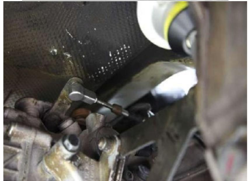
**#14. Connect the cables to the bracket inside the cabin but don't bolt it down yet and take the rod ends off the cables. This is so you slip the console back into position.**
