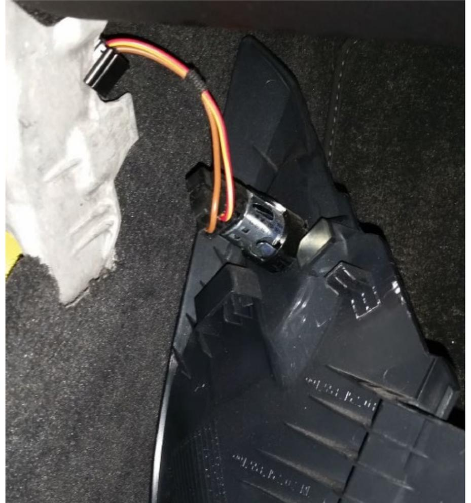
**#4. Remove the side trim pieces by pulling in the opposite direction for the front and they will snap out of place. The back is inserted into slots and you have to pull them out of the slots and then you can take them out.**
