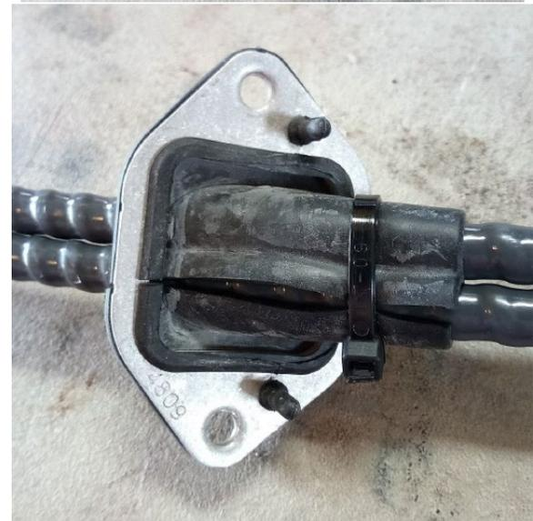
**#9. Next remove the rubber insulation and transfer to new cables. Cut it in a spiral so you won't need to zip tie it on. (Not necessary to use however recommended for noise reduction). Each car may be different, and you may or may not experience any noise. We also sell silicone tubing which you can insulate the cables with.**
