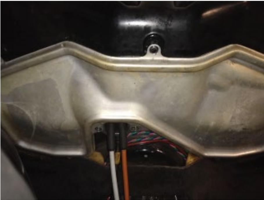
**#2. Next remove the tin over the engine. There will be several Torx bolts and be aware of the holes they came out of. They are different lengths.**
