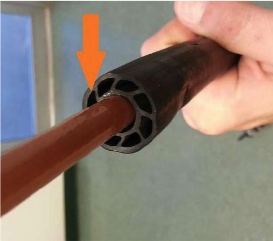
**#10. Now you will route the cables in the exact same way they came out. Slide them into the transmission brackets and into the shifter bracket. Do not connect any of the rod ends. Below are some examples. Models vary going over engine.**
