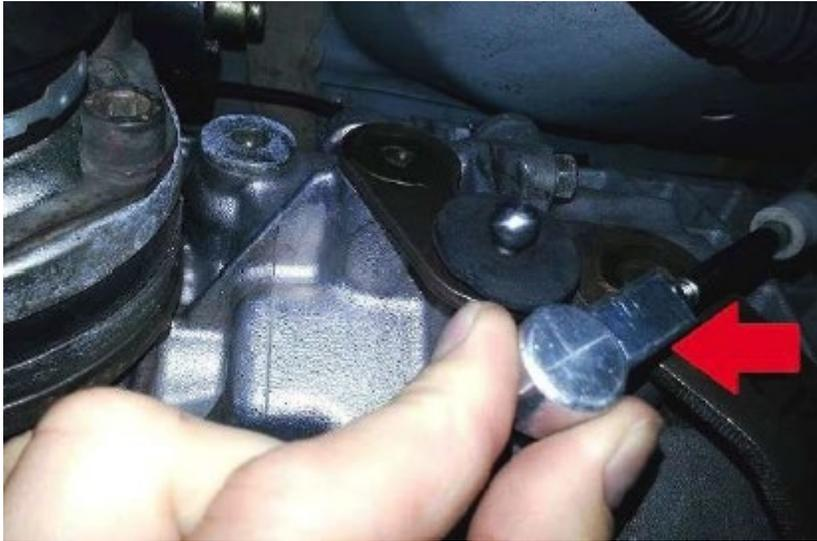
**#13. There will be a bag of 6 plastic inserts that came with the cables. These will always be attached to the balls on the transmission selectors first. Next, snap the rod ends onto the plastic inserts. If you have to break the connection make sure to use a new insert. Once it is adjusted properly lock the jam nuts in place.**
