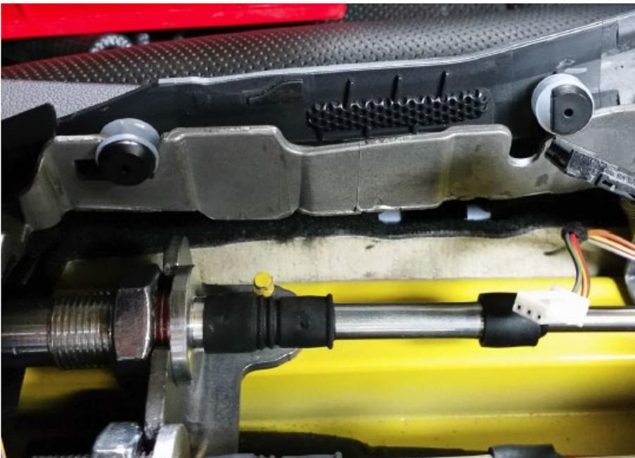
**#5. Next you need to remove the Torx screws hold the console in place. The will be (4) on the base of the console and there are several Torx screws holding the front in place.**
