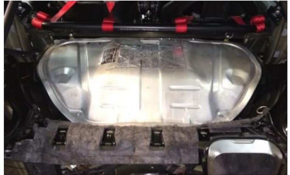
**#3. Next you will remove the front interior panels by removing the Torx screws. Push the panel forward to remove them from the slots.**
