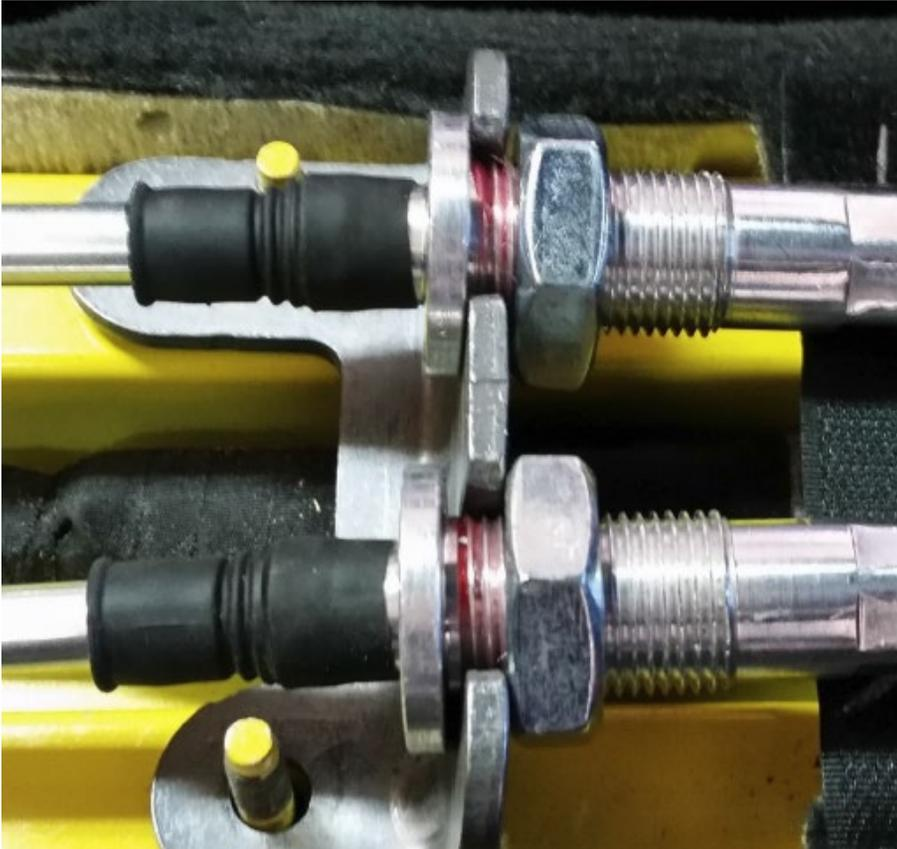
**#15. Now you need to slip the console back into place. It is a little tricky sliding it in over the cables. Make sure the longer cable (shift cable) is on the right side. Once it is in place reinstall the rod ends back onto the cable ends.**
