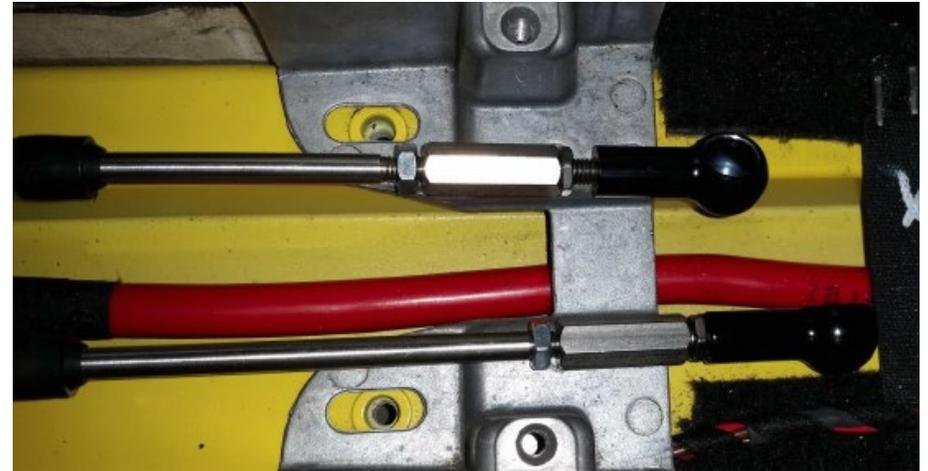
**#16. Now you need to connect the shifter onto the rod ends. Place the plastic insert onto the balls first then snap the rod ends on. For the left cable you will need to adjust the rod end to line up the mount holes for the shifter. Bolt the cable bracket on and tighten the 27mm nuts. Bolt the shifter down.**
