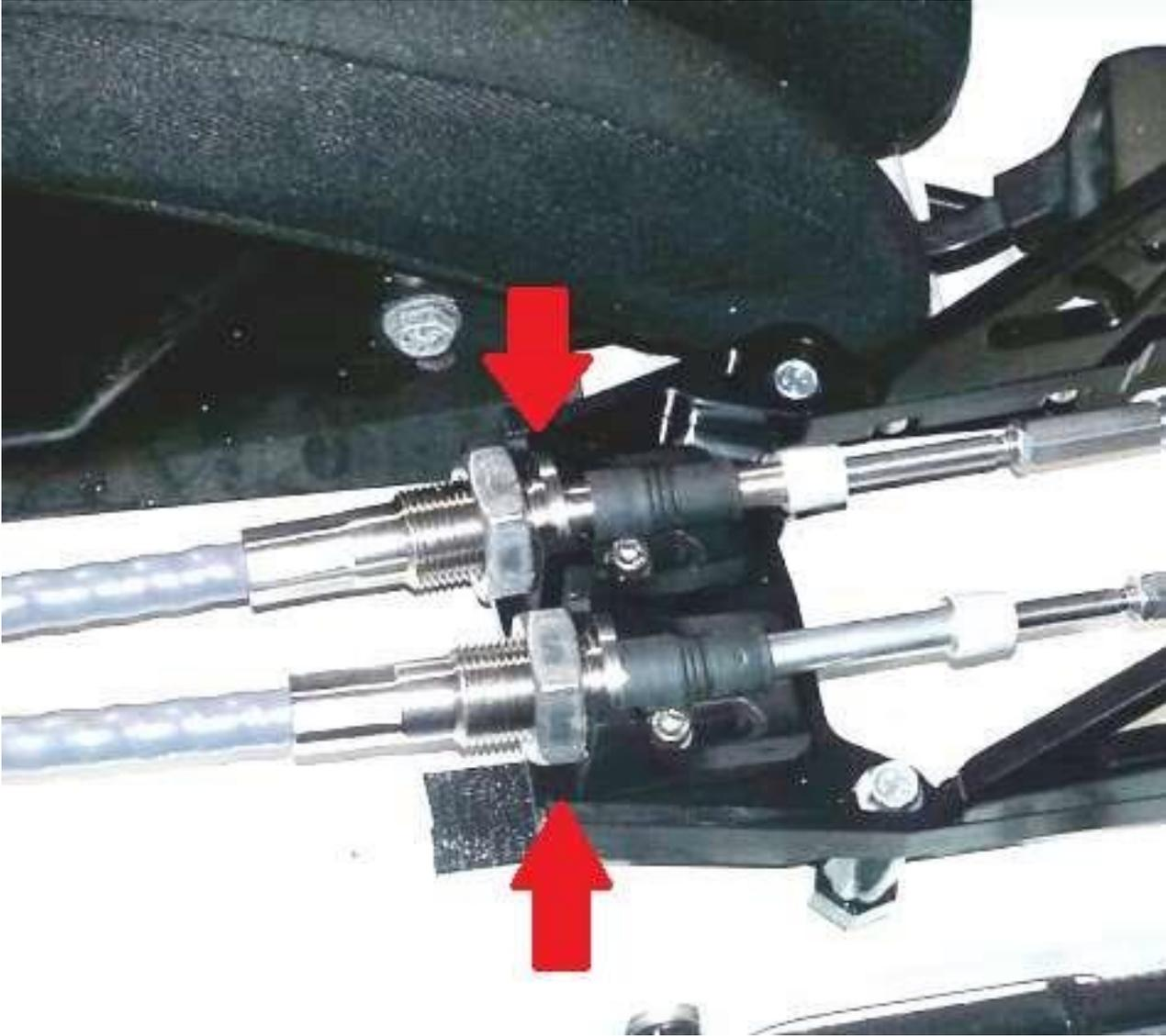
Note the right cable on the shifter will have the longer support tube.
