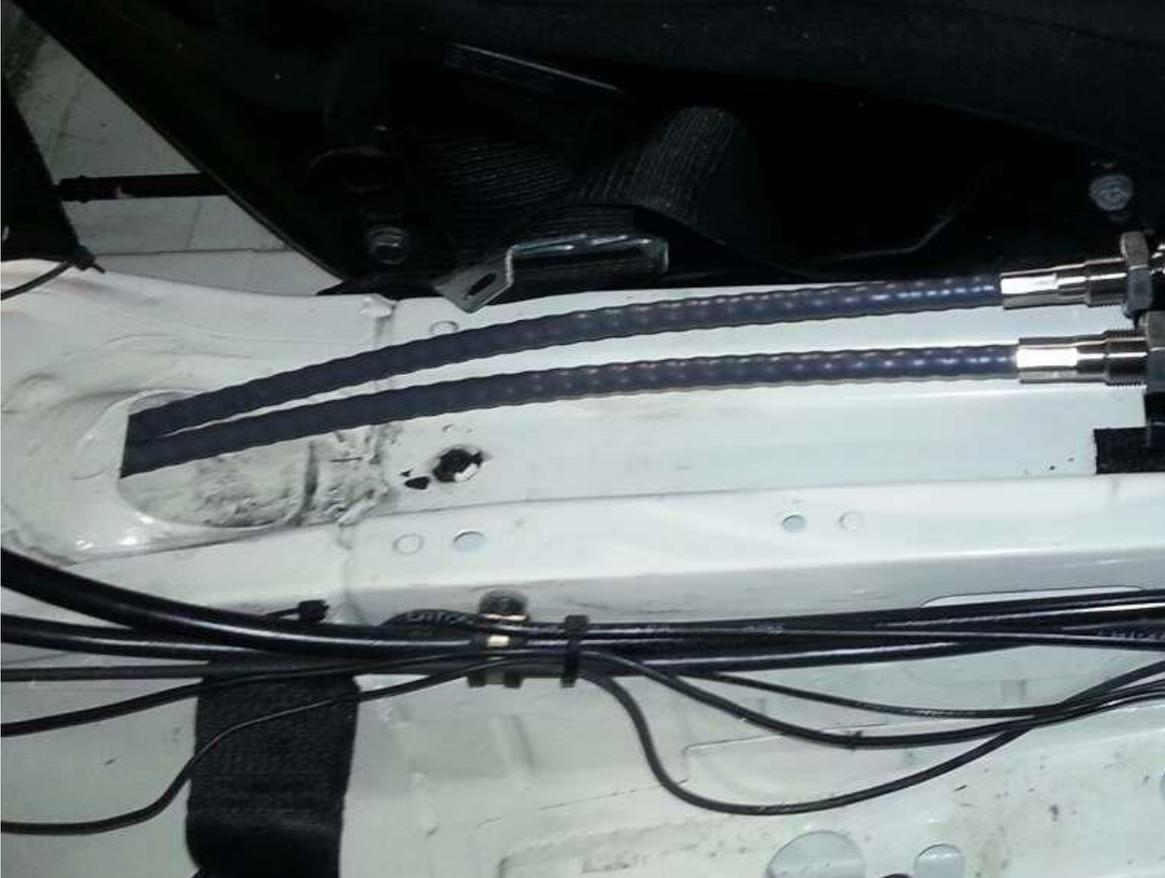
Example of the proper way to route the cables.
