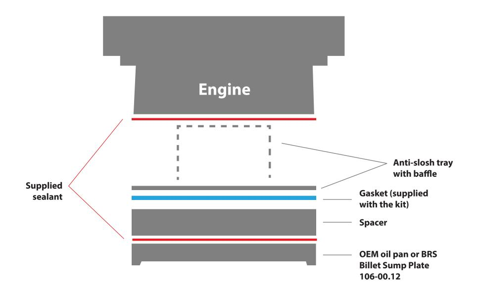
Starting with the OEM pan, remove the oil baffle. Clean the pan thouroughly. Remove the 3 baffle spacers from the packaging and set them in location on top of where the OEM baffle was fastened.
