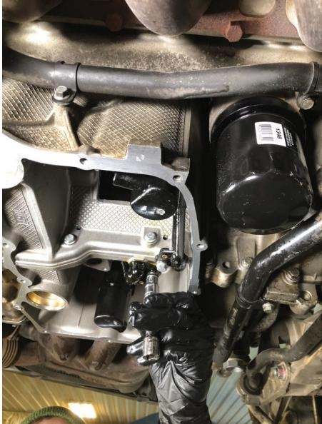
(Continued) Remove the oil pickup, and the oil swirl pots. The swirl pots will be replaced by the revised 997 versions from Porsche. The BRS 2qt Deep Sump kit cannot be installed with 996 swirl pots.
