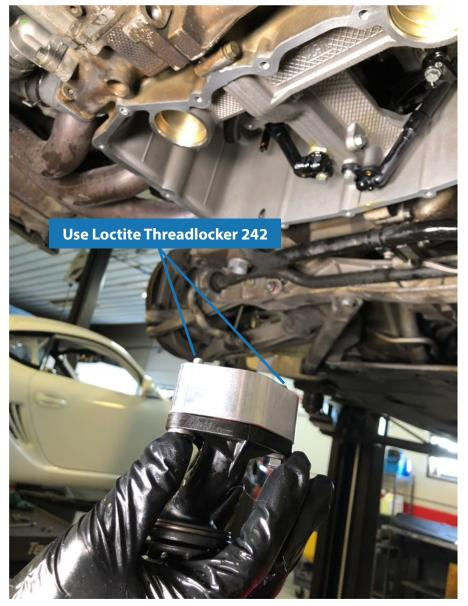
Properly installed pickup spacer and oil return tubes shown below. Ensure all fasteners are torqued to factory specs.
