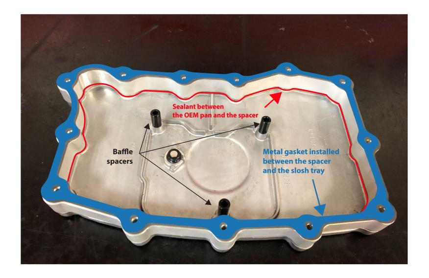
Set the flat anti-slosh tray on top of the assembly. The baffle can now be placed on top and properly fastened. Please use the Loctite Threadlocker 242 on the baffle fasteners. Using the supplied sealant place a smooth bead on top of the windage tray. Ensure the sealant completely surrounds the fastener locations. Orange silicon edge strips must be installed to prevent baffle from rubbing on inside of engine sump.
