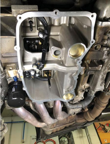
Next, to ensure the oil pickup is properly submerged in the extra capacity of oil the provided spacer must be installed. Note that the o-ring on the pickup is mated to the flat side of the spacer, and the o-ring side of the spacer is mated to the block. Please use the Loctite Threadlocker 242 on the pickup spacer bolts.
