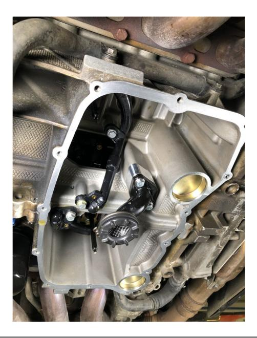
Now we are ready to prepare the sump and baffle for installation. Proper order of the deep sump kit components:
