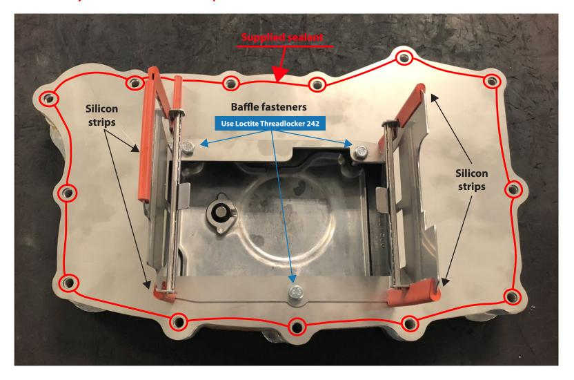
With the sealant applied place it up to the engine and begin to add the fasteners. DO NOT USE the Threadlocker 242 on these bolts. Torque to factory spec.
