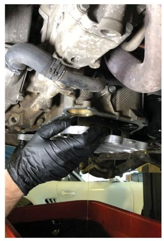
Remove the oil pickup, and the oil swirl pots. The swirl pots will be replaced by the revised 997 versions from Porsche. The BRS 2qt Deep Sump kit cannot be installed with 996 swirl pots.
